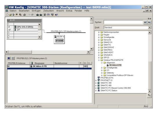
Allocate the correct Profibus address of the module.
