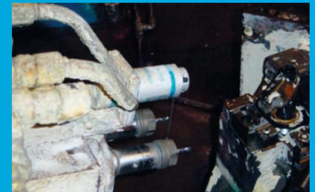
Tool breakage inspection: Bidirectional scanning
