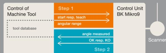
Instructions and parameterization data are transmitted from the PLC to the control unit. Reversely, the control unit sends its status reports to the machine control.
