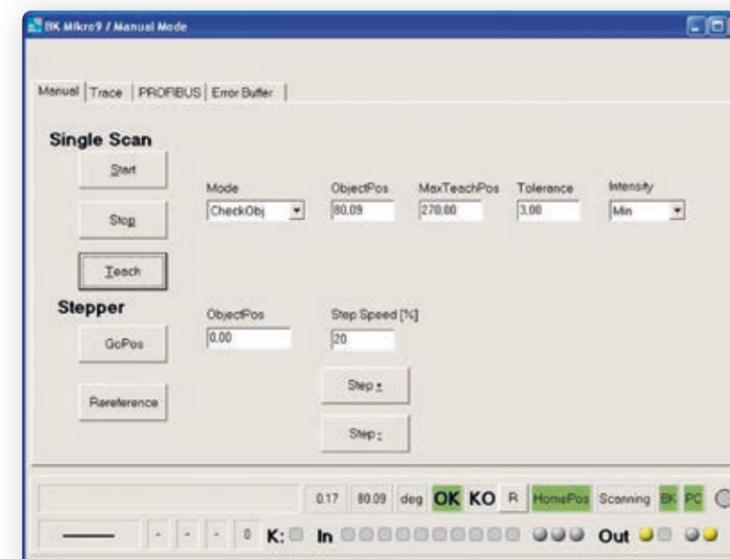
“Scan” manual mode attribute: For quick monitoring and displaying of angles, tolerances and intensities.
